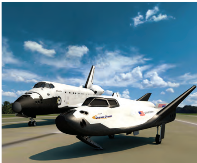
The lifting-body design of Sierra Nevada Corp.'s Dream Chaser enables it to potentially land on any commercial runway and draws comparisons with the space shuttle. Image courtesy of SNC.
